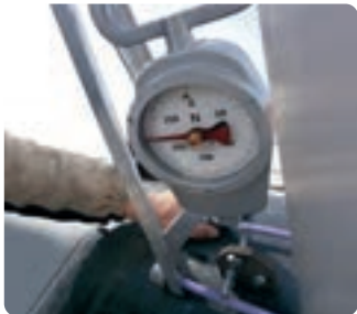
Adhesion test of ANTICORRay® WSS60 heat shrink sleeve
