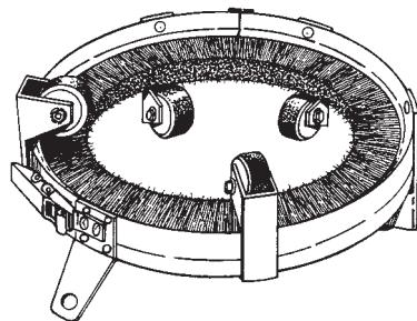
60mm, 125mm, 200mm, 450mm **connectors** for flat or external pipeline brushes.
